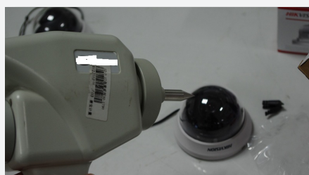
Test device for electrostatic discharge anti-interference
