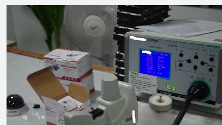
Test device for electrostatic discharge anti-interference
