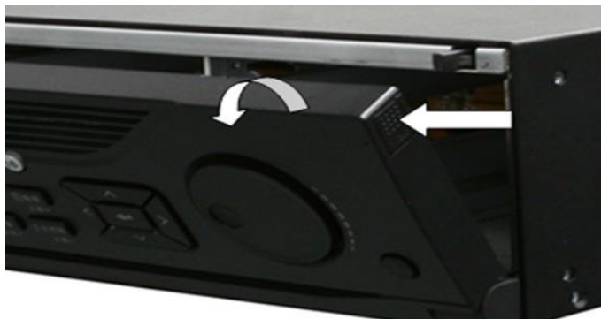
Figure 2-3 Open Panel Lock
