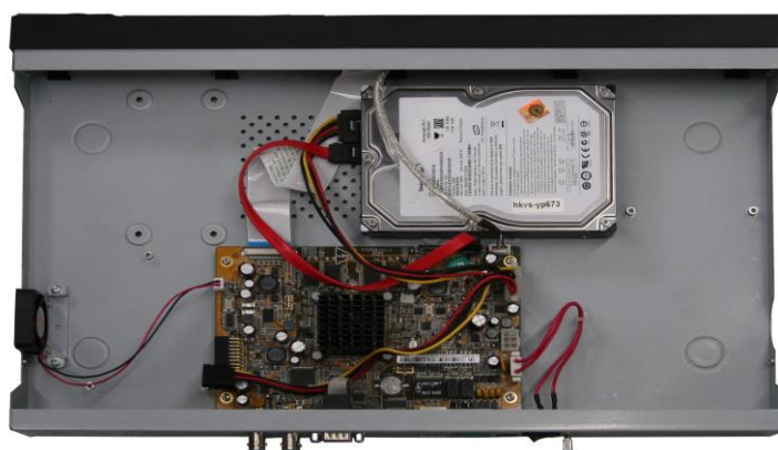
Figure 2-9 Fix Hard Disk
