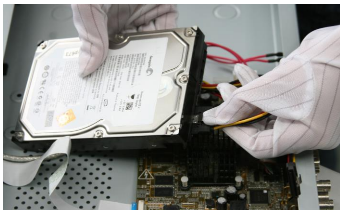
Figure 2-8 Connect Power Cable
